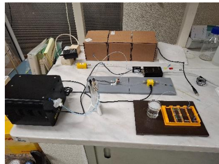
Figure 1 – Flow resistivity setup with a pressure-driven generator.
