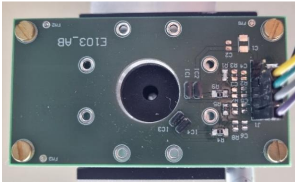
Fig. 2: Backside of circuit board of the sensor with two radial Hall-sensor pairs assembled by INNOVENT, [2].
