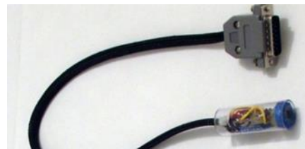
Fig. 4. The basic probe without positioning sensor.
