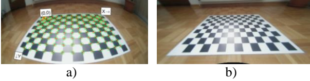
Figure 1 Calibration process (a) distorted image and (b) calibrated undistorted image.
